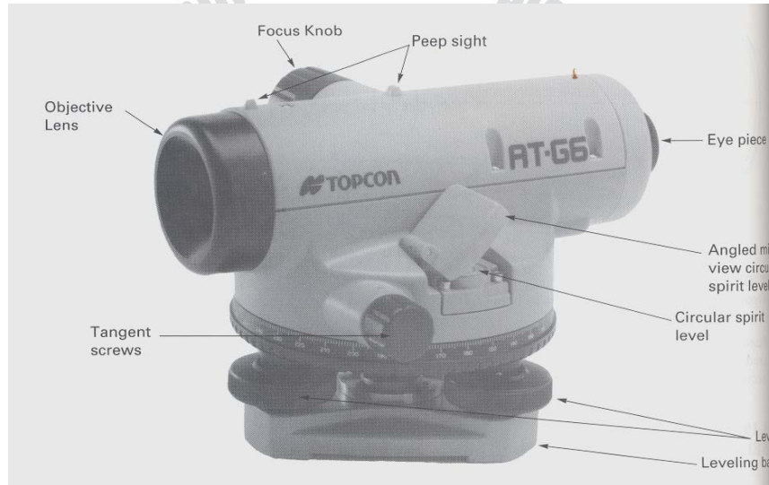
Fig 5.6. Automatic Levels
